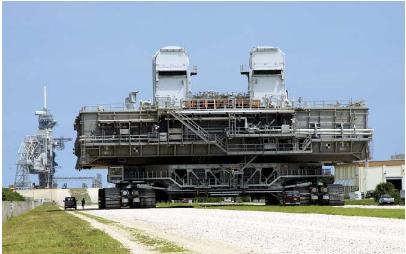
A Mobile Launcher Platform makes a test run to the launch pad. Rising above the MLP are the tail service masts.
