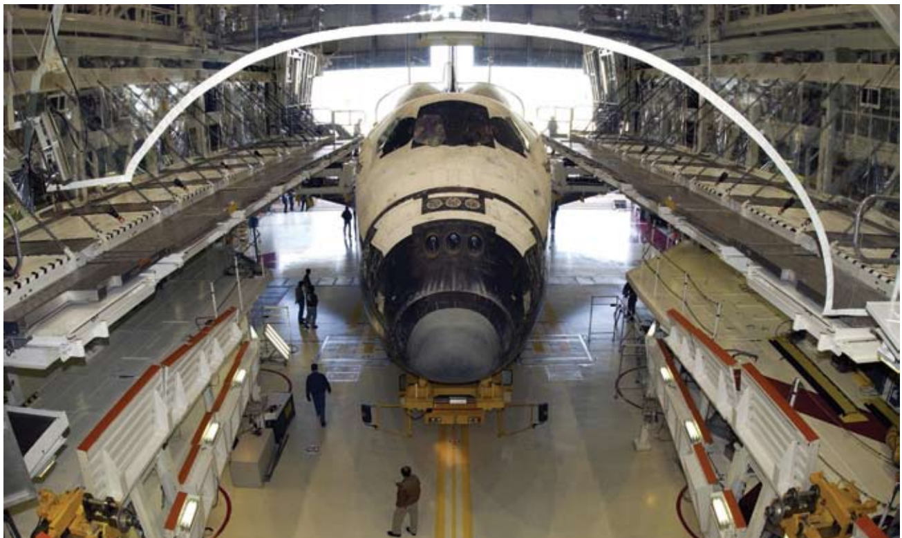
Processing for a mission begins when an orbiter is towed into one of three Orbiter Processing Facility bays at KSC.
