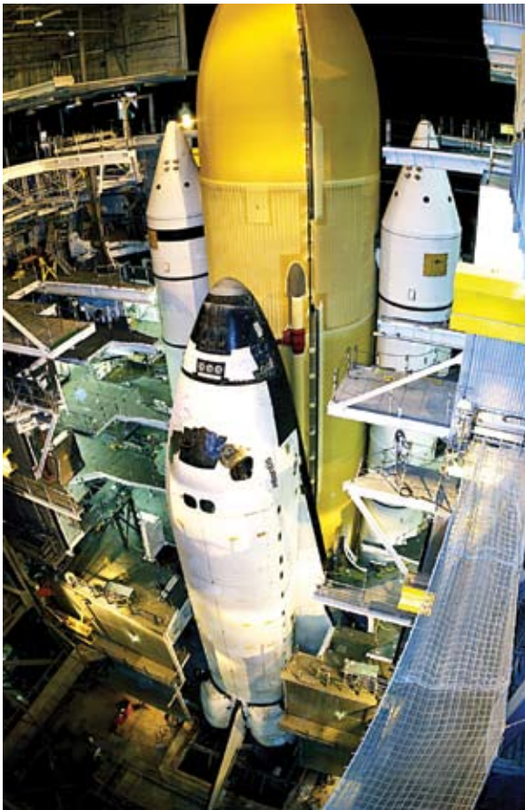
Atlantis is in the Vehicle Assembly Building where it has been stacked with the orange external tank and solid rocket boosters.
