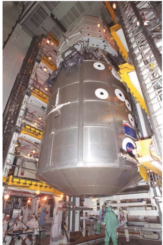
Two payloads – the Canadian robotic arm or Space Station Remote Manipulator System, and the Multi-Purpose Logistics Module Raffaello – are moved into the Payload Changeout Room for mission STS-100.
